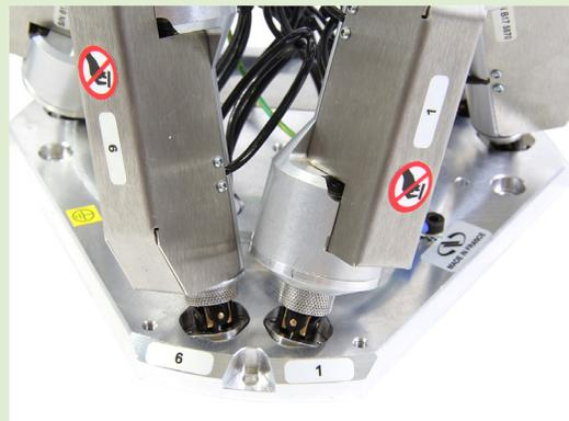
What distinguishes of the HXP50, as with the other Newport hexapods, is the ability to program two pivot points represented by the Tool and Work coordinate systems. The Tool CS moves with the top plate and the Work is stationary. Imagine a machine tool where one can adjust the orientation of both the cutting tool and workpiece or in photonics, the optical beam and the
